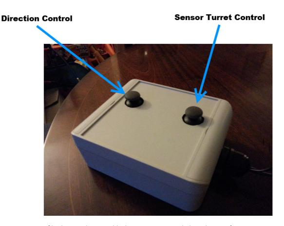
Concurrent operation of both controls is possible, but not recommended. For best performance, stop TempEx before steering the sensor turret. Do not move the turret control rapidly – wait for a command input to be answered (i.e., wait for the turret to move) before giving another.
