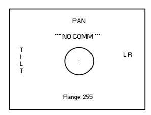
The pan and tilt indicators display the command inputs from the turret control. The LR indicators display the command inputs from the direction control. Range to target is shown in centimetres at the bottom of the display; if this reads 255, the target is either out of range or is not perpendicular to TempEx. NO COMM is displayed if the controller cannot communicate with TempEx.
